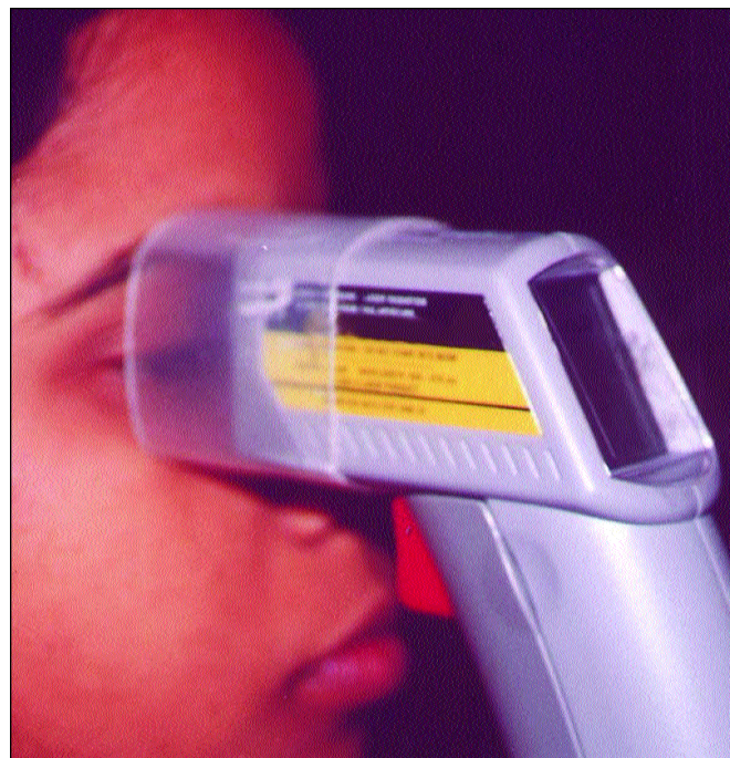
Fig. 2 - Recording thermometer for infrared thermometry with a silicone closed chamber fitted on the mouth of the thermometer.
